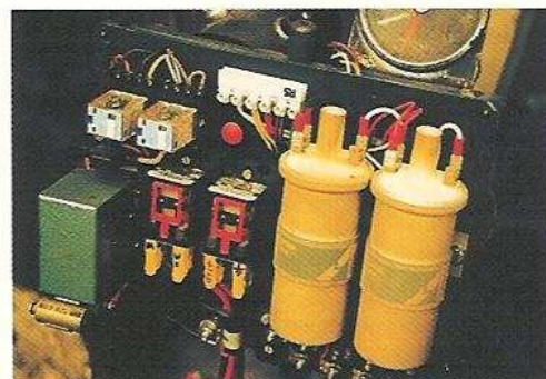
The electrical control panel of the Dolphin Direct Drive engine (above) and a cut-away showing the ignition system in place (right)
