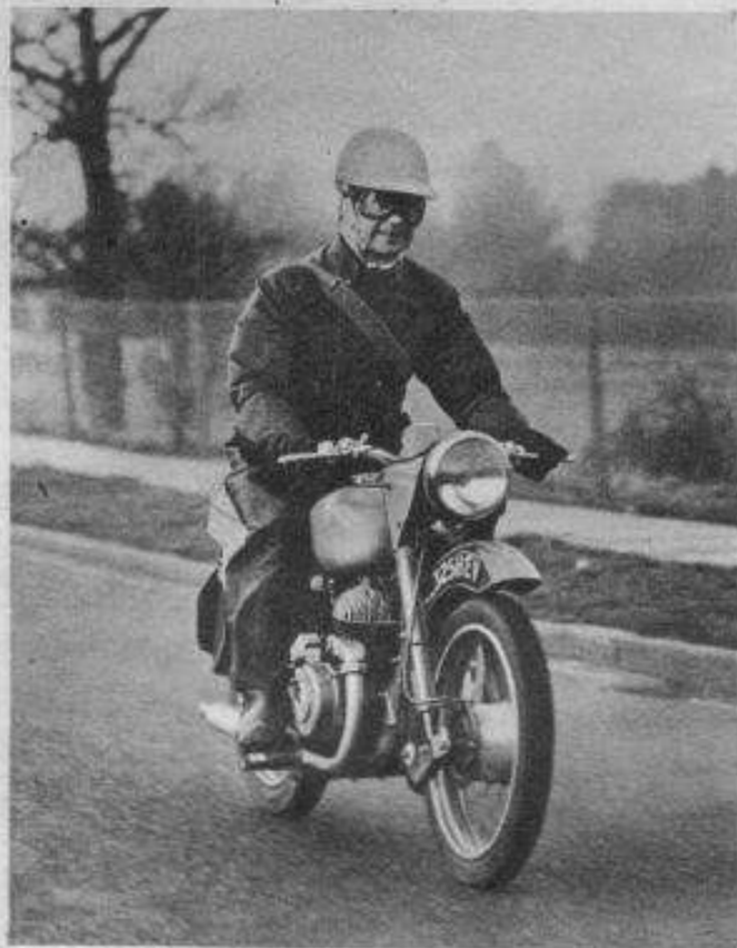
Predominant trait of the RCA engine is its wide spread of high torque. Acceleration is smooth and brisk from idling speed upward. Below: Two Amal carburettors and a 12-volt Siba Dynastart are fitted
