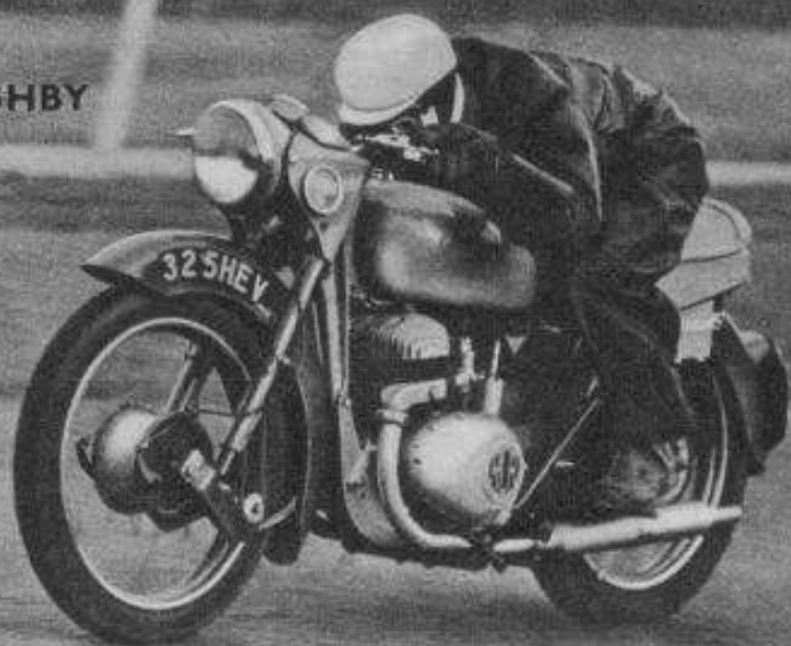
Ridden in this fashion, the RCA-engined Greeves is timed at 78 m.p.h. in one direction; mean maximum speed was 76 m.p.h.
